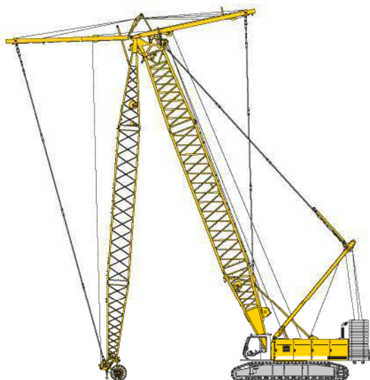
Erecting of main boom and luffing jib
