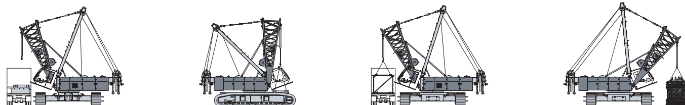
Unloading and assembly of carbody counterweight
