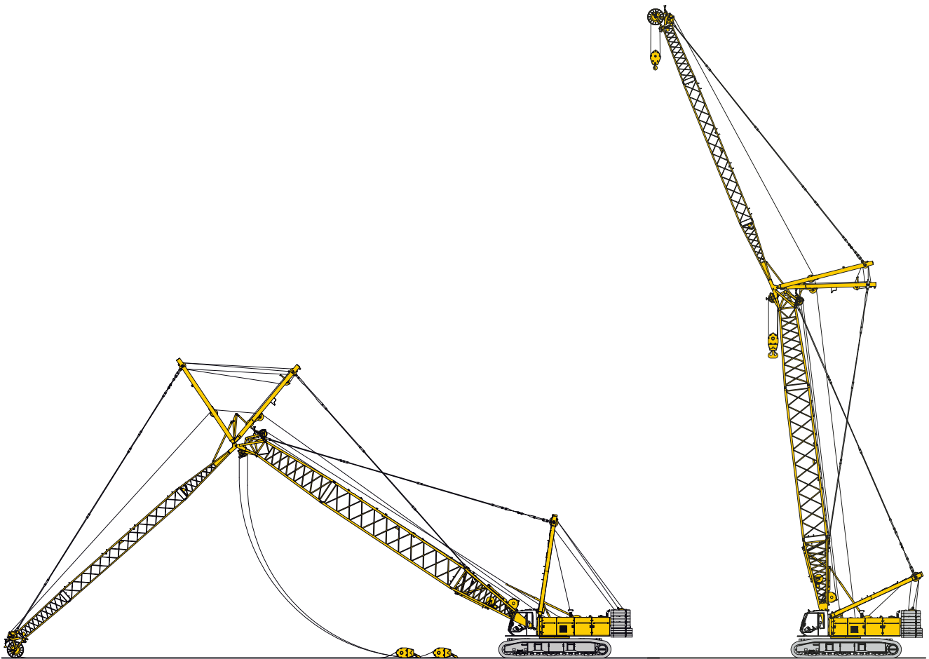
Erecting of main boom and luffing jib
